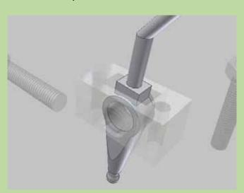
The new finger fit into the receiver on the main shift plate (yellow arrow), This must be measured and arranged on the shift plate and then welded.
