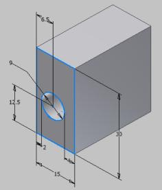
$\leftarrow$  Two (2) 30mm  $\times$  30mm  $\times$  15mm piece with a 9mm bore
