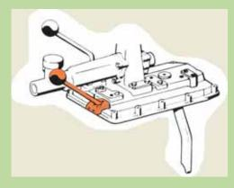
You could modify the inner pivoting arm for the fwd / reverse lever (II on page 7) and have this to actuate the high/low range and use it instead of the additional shift lever for forwards and reverse selection More than only one way to go for sure.
