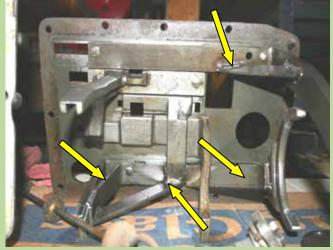
Most of the modification is to be done here on the shift plate, and consists more or less in taking pieces away .
