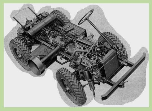
Note the lateral power take off with a big pulley for belts or hydraulic pumps and the early type shift covers...
