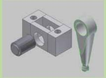
Now fabricate a receiver piece for the shift lever:  $(16\text{mm} \times 12.5\text{mm} \times 8.5\text{mm})$ , the bore is centered).  $\rightarrow$
