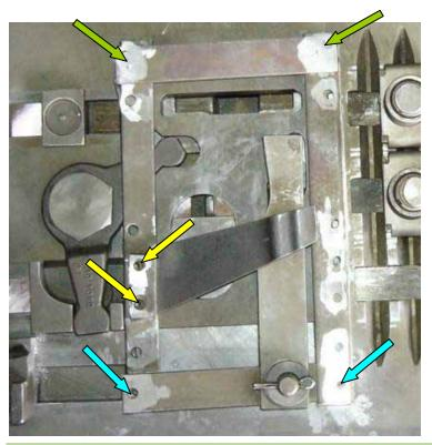
With a small grinder or a "Dremel" grind the yellow arrowed rivets careful away, take the small plate and the (black) holder apart. Then grind the two light blue rivets away and take the little traverse with the lock arm (complete) apart. Help with a small flat sharp chisel and a hammer to separate the pieces. Take the slide plate out.
