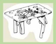
Second, put the shifting plate on the bench or grip: When you have the part cleaned and ready: To manipulate the shift plate easier, put the springs and associated parts from the fwd/rev and from the high/low range detent apart for a while.
