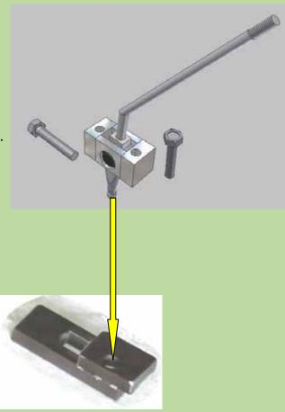
The counter part to actuate the high/low slider on the shift plate is made of the two pieces cut from the shift fork (s. page 13).
