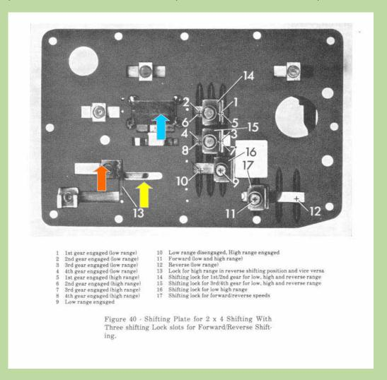
There is one minor difference on this plate, it is the little slot above the #13 (arrowed yellow), this could be used to shift the high/low range where it is already present if you have this version of the plate from a newer (2x4) transmission and the lever with the longer finger. If this is your case, you need to make a lever with aprox. an 80mm long finger.
