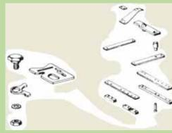
Here is a shift plate from an UG2/27 tranny. Same size, same holes and bores, the slots for the engaged position of the shift forks. Compare !, it is the same basic plate, - fundamentally.
