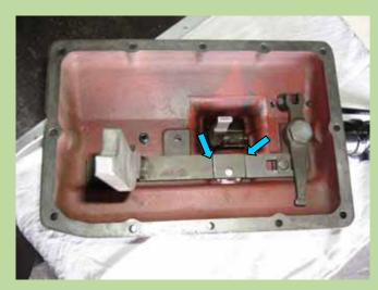
When the shifting fork is apart, mark 75mm (from the right to left) and a second segment of 40mm. Cut the pieces and eliminate sharp edges, sand them. This pieces are for the connection of the new shift lever with the high/low range slider on the shift plate.
