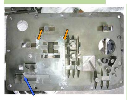
You can punch these two rivets out to the other side. The others can be left in place, due to its shape they can not fall out and the sliders hold them from the other side. If you want, spot weld them. Cut the square shaped pin of the security lock of the reverse gear (grey, w. blue arrow).
