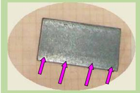
Smooth and polish the surface where the finger of the main shift lever will slide along.
