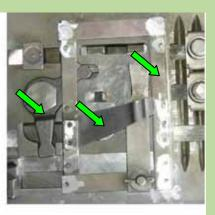
The angle lever for the 'Q' - shifting of the high /low range in the  $1^{st}$  and  $2^{nd}$  gears forward and reverse, the flat holder, the frame with all its components and the slider plate- are not needed. You can save them as spares (or elaborate a trophy for the next NWMF .....?).
